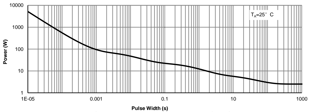
Figure 14: Single Pulse Power Rating Junction-to-Ambient (Note H)
